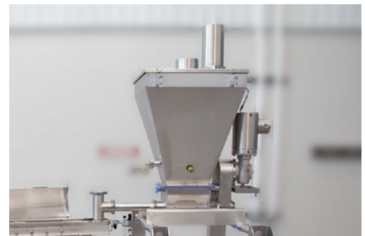
Adaptable hopper and lid assembly compatible with a variety of mechanical or pneumatic refill options.
